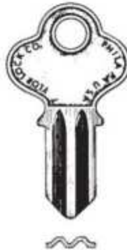
Figure 6.17 Four basic double-bitted key sections. ( Taylor Lock Company )
