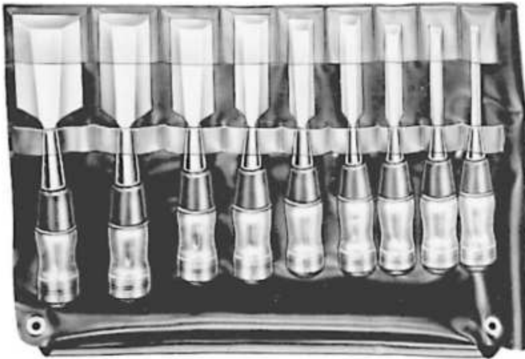
Figure 2.39 Wood chisels of various sizes are needed when installing locks and other hardware on wood doors. ( Stanley Works . )
