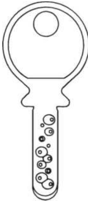
Figure 8.18 Eleven oblong bit-tings equal Kaba Gemini. ( Lori Corp . )
