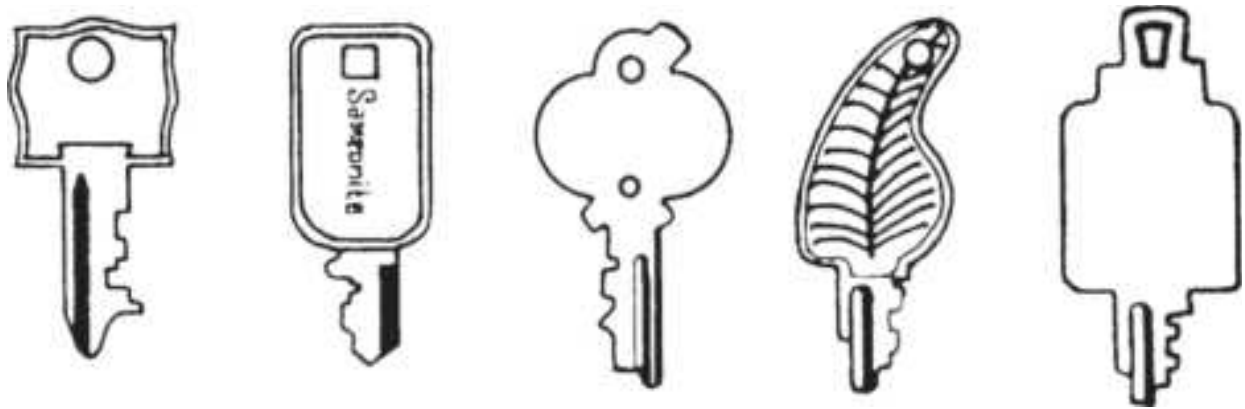
Figure 5.20 Typical flat key blanks used to make keys for lever tumbler locks.
