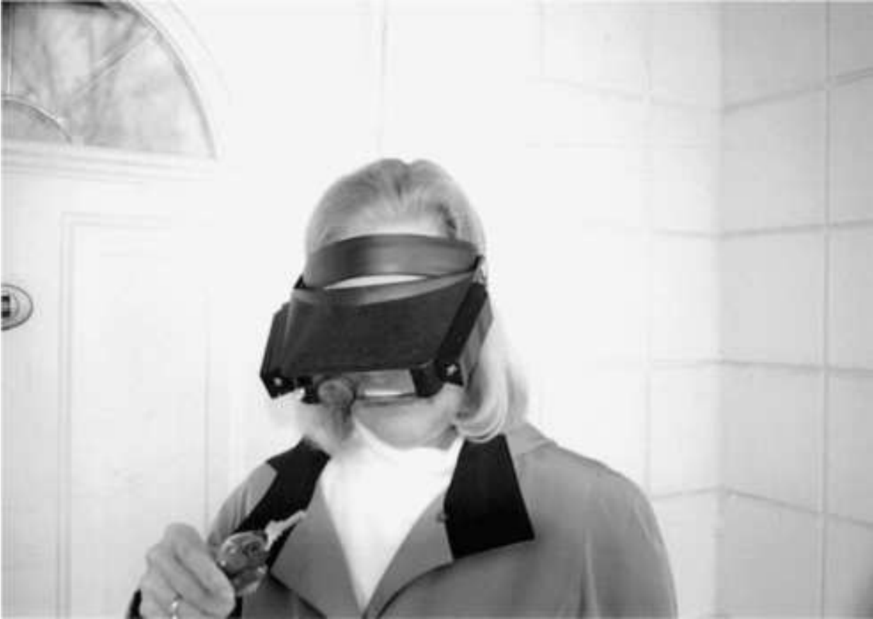
Figure 14.14 Head-mounted magnifying glasses can help you to see impression marks.
