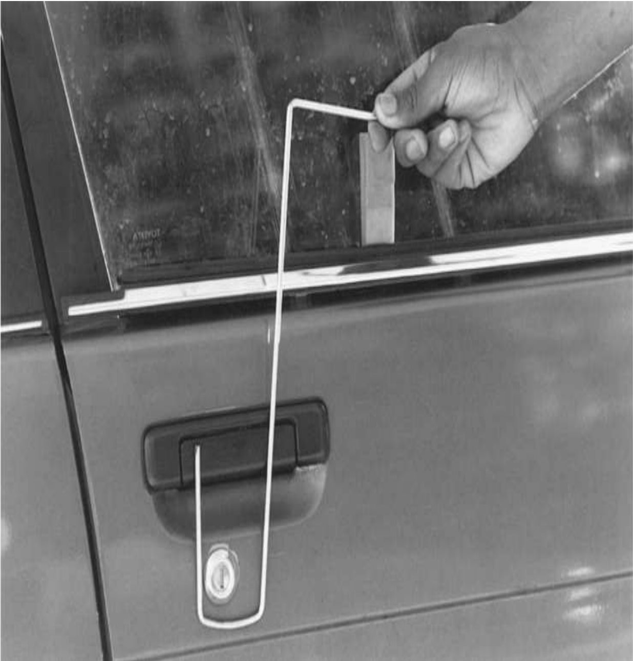
Figure 16.6 A J tool shown outside the car. The tool goes beneath a lock button and pushes it up to unlock a vehicle.
