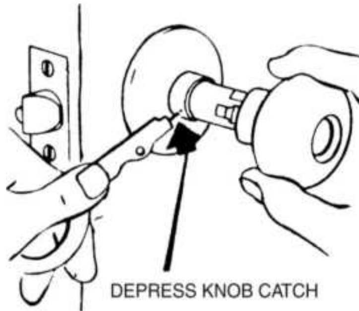
Figure 19.50 Electrified key-in-knob lock installation, Step 7.
