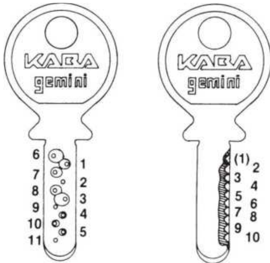
Figure 8.10 Positions on Kaba keys. ( Lori Corp . )
