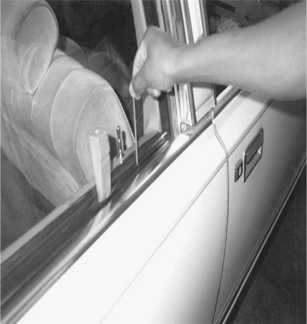
Figure 16.11 When the J tool is below the window, turn it so it is beneath the lock button.
