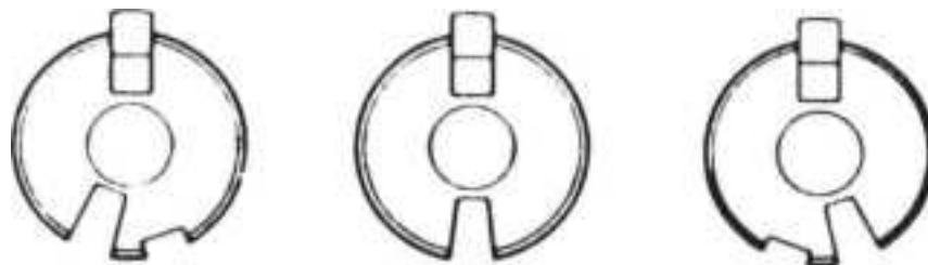
Figure 8.30 The locator tab is located along the centerline of the Medeco biaxial pin opposite the area for sidebar slot. ( Medeco Security Locks )
