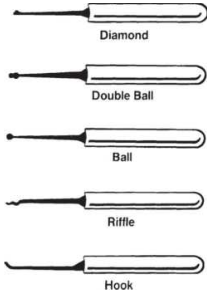
Figure 2.17 A variety of lock picks allow the locksmith to choose the best one for a given lock. ( A-1 Security Manufacturing Corp. )
