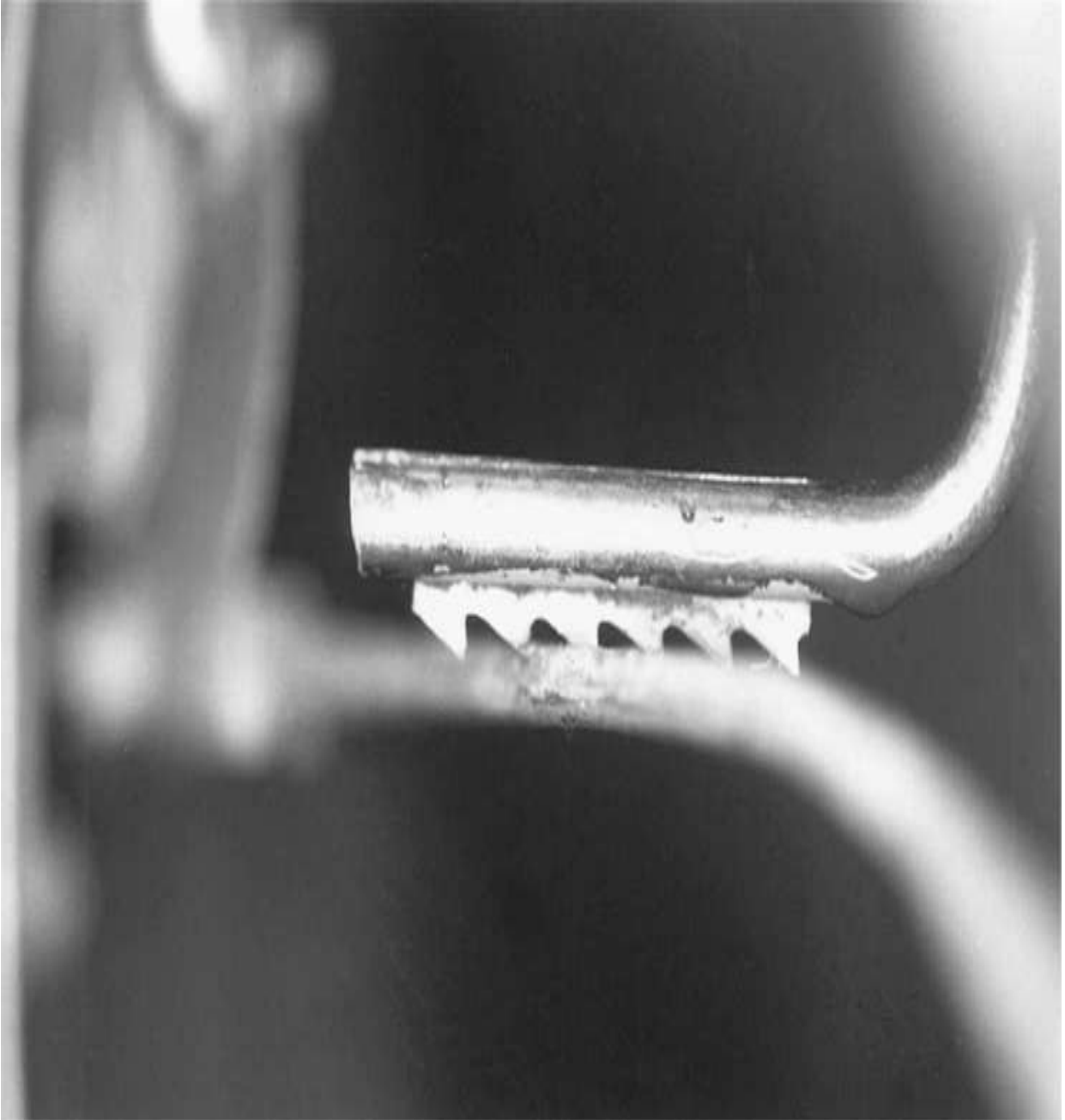
Figure 16.5 A car-opening tool with teeth grips a rod by biting into the metal.
