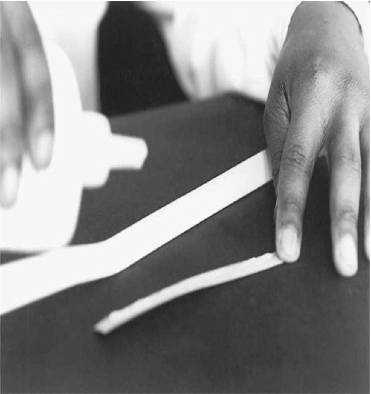
Figure 16.16 Glue a piece of sandpaper to the center.
