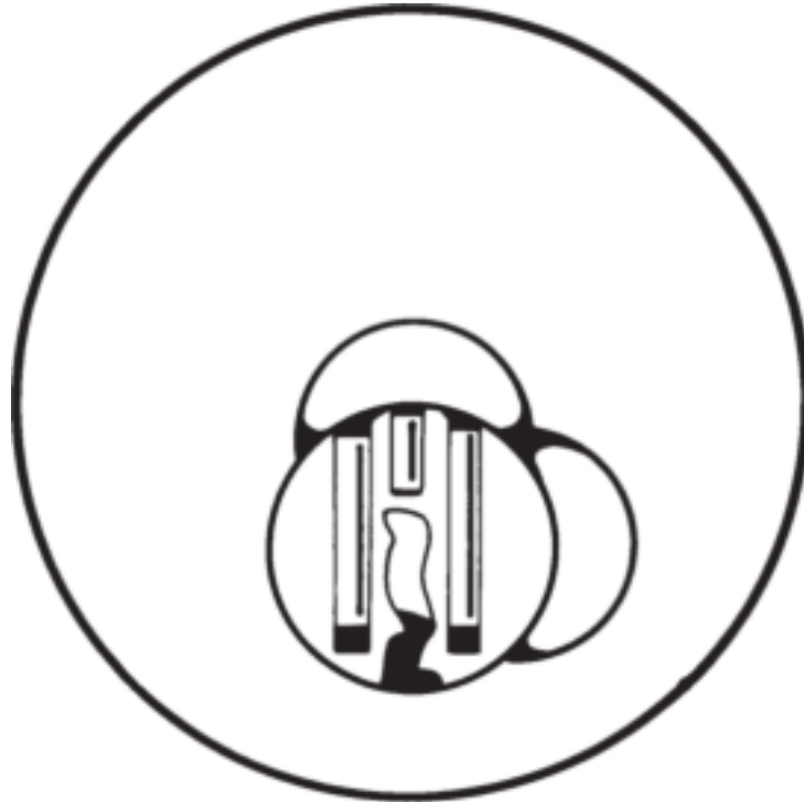
Figure 8.22 Face of a Medeco cylinder showing the positions of the hardened steel drill-resistant pins and crescents. ( Medeco Security Locks )
