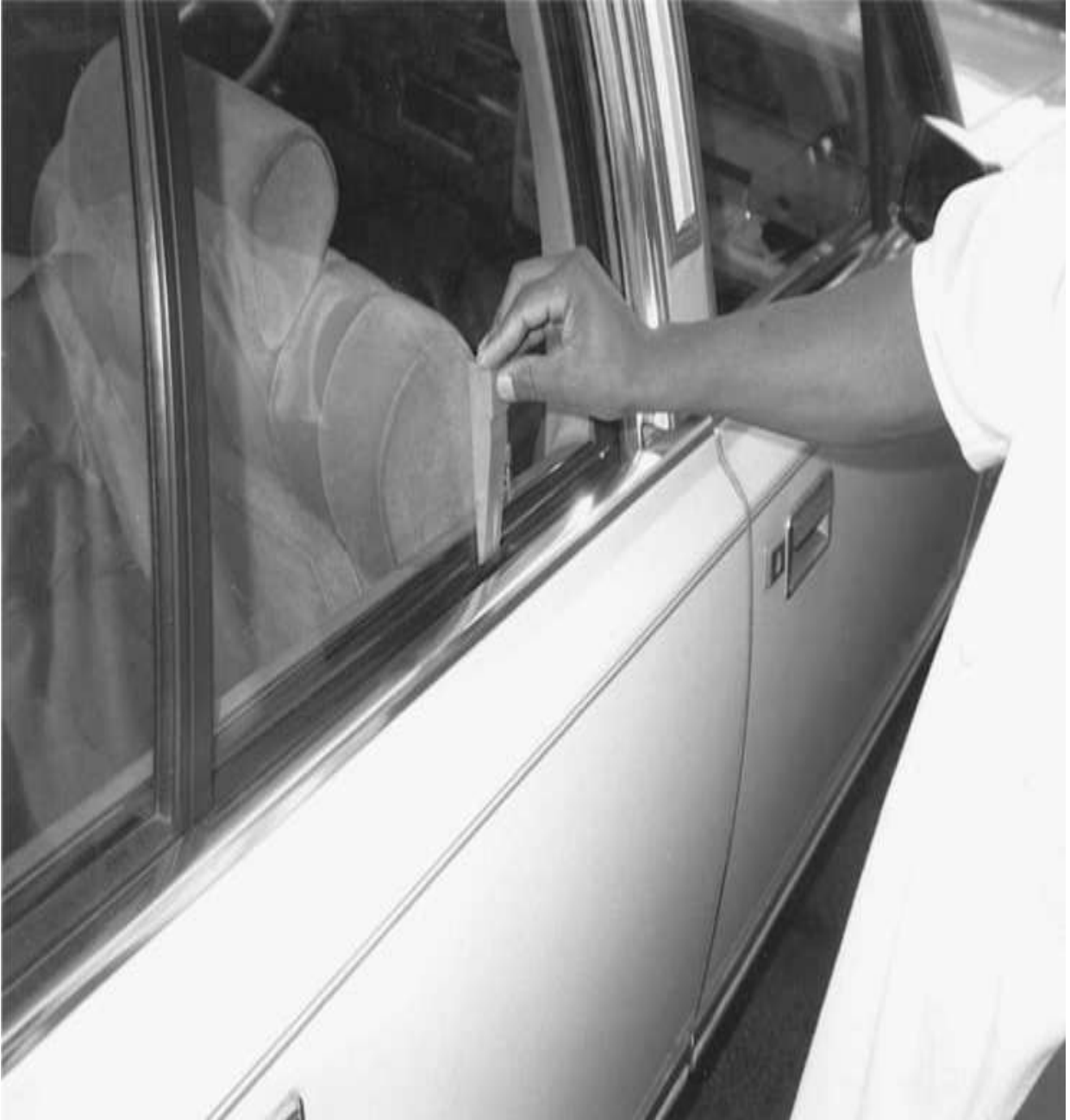
Figure 16.9 Before inserting a tool within a car door, insert a wedge to spread the door a little.
