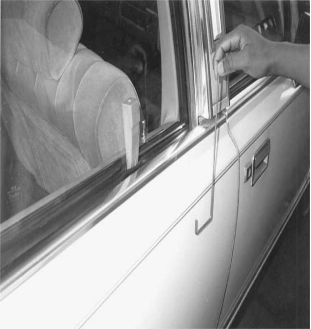
Figure 16.10 The J tool goes within the door near the lock button.
