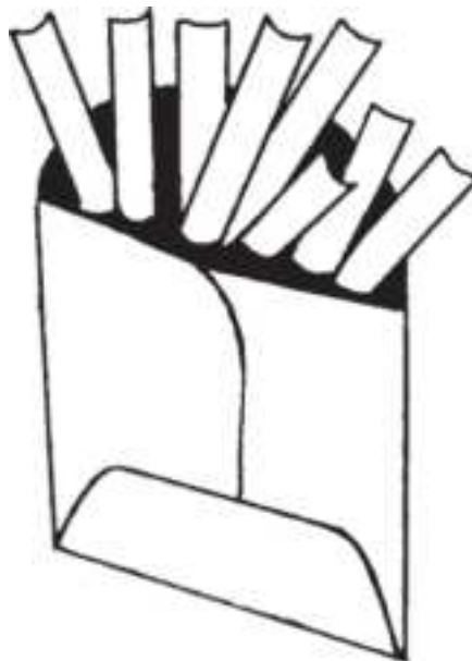
Figure 2.24 Shims are used when disassembling pin tumbler cylinders. ( //co )
