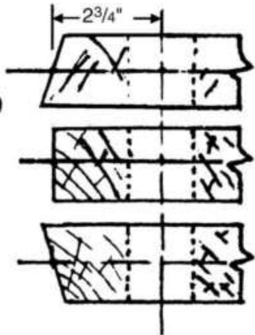
Figure 18.32 Unican 1000 latch cutout specifications. ( Simplex Access Controls Corp. )
