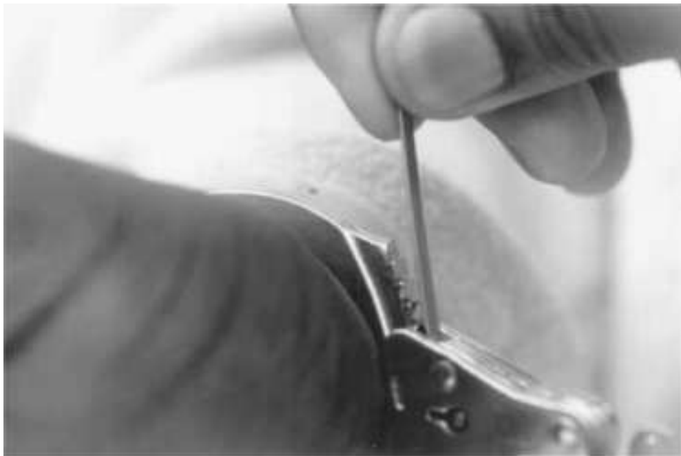
Figure 17.15 Place the shim between the ratchet and pawl to open cuffs.
