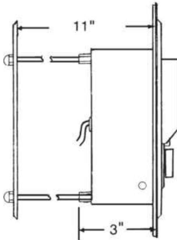
Figure 19.65 Lock unit can be mounted on any thickness wall up to 11 inches. ( Simplex Access Controls Corp . )
