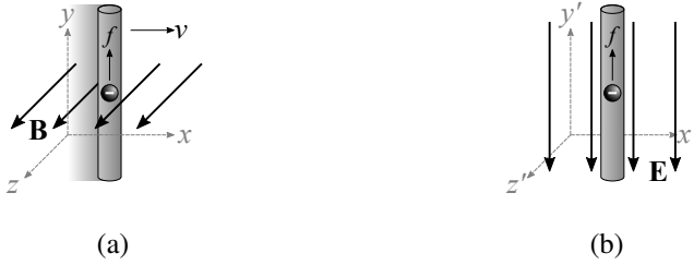
Figure 4.3 Transformation of the electromagnetic field tensor. (a) An electron in a y -directed wire moving in the x direction through a z -directed magnetic field, \mathbf{B} , experiences a force in the positive- y direction. (b) The same force in a reference frame that is comoving with the wire must be due to an electric field, \mathbf{E} , instead, since the electron starts apparently at rest.
