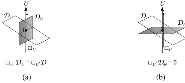
Figure 6.2 Illustration of vector-projection product identities. (a) The tangential divergence of a bivector field projected onto the same vector as the derivative is equal to the tangential divergence of the field as a whole. (b) The tangential divergence of a bivector field rejected from the vector along which differentiation occurs is zero.
