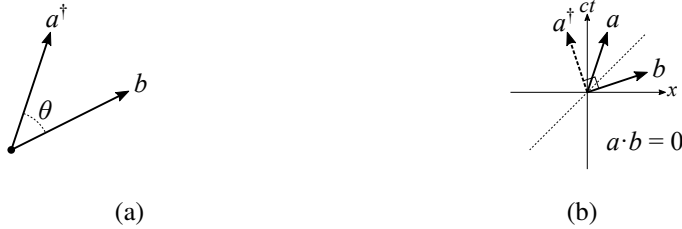
Figure 5.3 (a) The dot product measures the magnitude and colinearity between two vectors. (b) Dot products in Minkowski space must account for the metric signature; two vectors can be orthogonal in Minkowski space without appearing to lie at right angles in Euclidean space.
