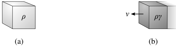
Figure 4.1 (a) A cubic lump of charge density, \rho , at rest. (b) The lump of charge in motion, having a new density, \rho\gamma = \rho \cosh \zeta , due to Lorentz contraction of its spatial distribution.
