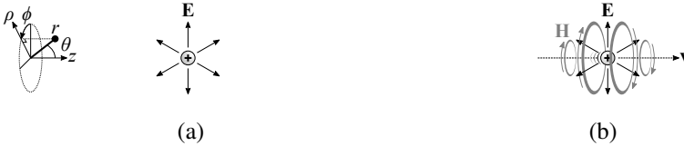
Figure 4.4 Emergence of the magnetic field as a dynamic correction to the fundamental Coulomb force. (a) Electrostatic field of a stationary point charge. (b) Transformation to a reference frame in which the charge is seen to be moving reveals an emergent magnetic field.
