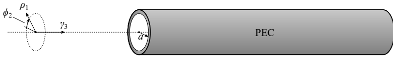
Figure 7.3 Geometry of a circular waveguide and the system of cylindrical coordinates that will be used to describe it.
