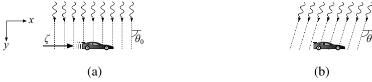
Figure 3.2 Illustration of relativistic aberration using the analogy of a car driving through the rain. (a) The rest frame, in which the rain falls vertically. (b) In the driver's reference frame, the rain appears to slant toward the car.
