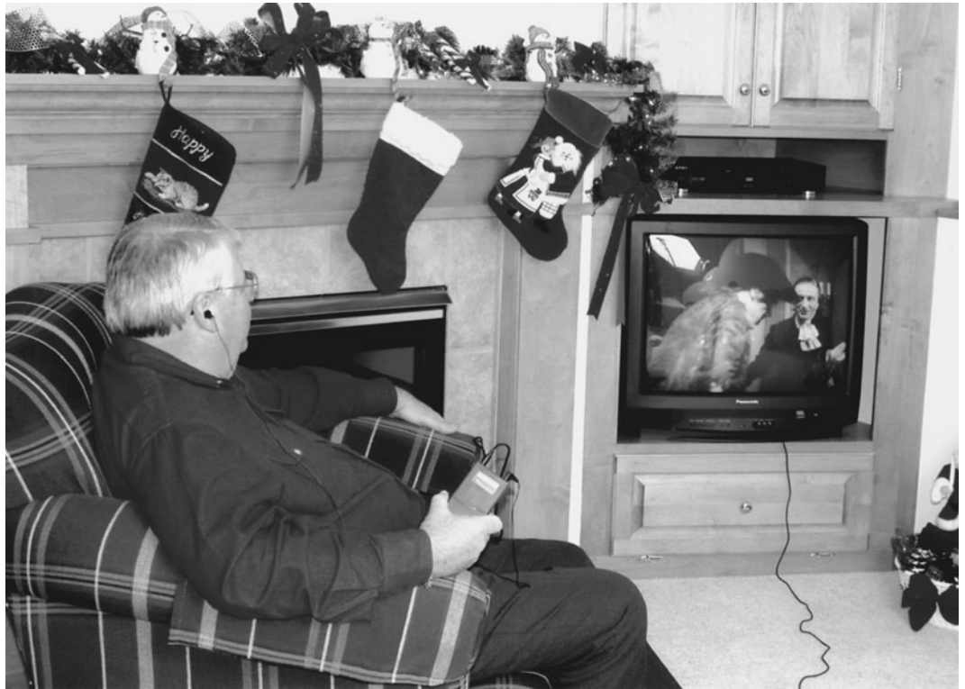
FIGURE 14.18 A “personal communicator” amplifier to enhance communication in the absence of custom hearing amplification. The device may be plugged directly into the television set or other audio-output jacks to provide direct sound to the user’s ear thereby improving the signal-to-noise ratio. With a plug-in microphone, such devices can also be invaluable in helping to maintain more private conversations between healthcare providers and their patients in compliance with privacy legislation. (Courtesy of Williams Sound Corporation)
