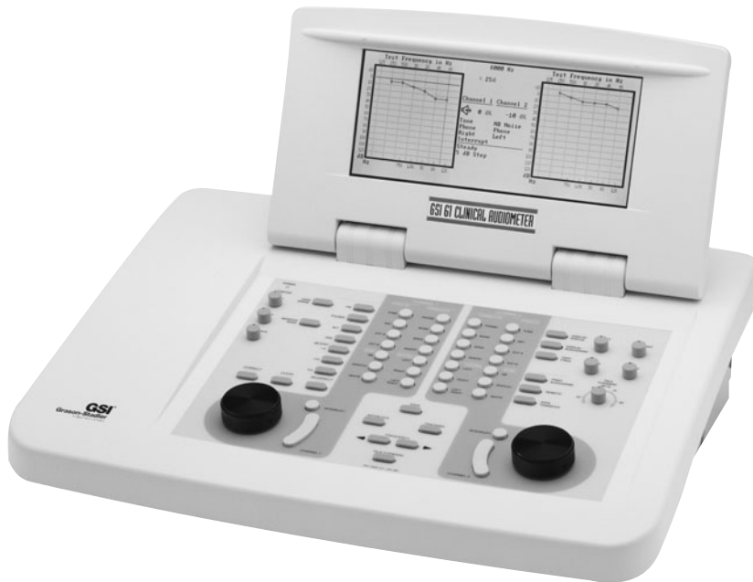
FIGURE 3.23 A diagnostic audiometer measures hearing sensitivity for speech and for tones via either air or bone conduction. (Courtesy of Grason-Stadler Co.)
