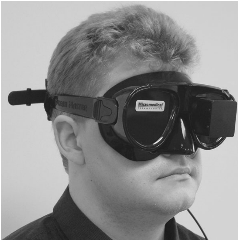
FIGURE 11.2 Specialized goggles allow for the observation and video recording of eye movement while testing the dizzy patient or while performing vestibular rehabilitation. (Courtesy of Micromedical Technologies, 10 Kemp Drive, Chatham, IL 62629)
