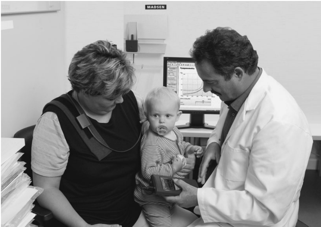
FIGURE 7.1 An electroacoustic immittance meter for the assessment of middle-ear function can measure the mobility of the tympanic membrane, the air pressure within the middle-ear cavity, and the presence of the acoustic reflex. Bluetooth wireless technology allows transmission of collected data to be sent to an off-ice computer for storage and printing. (Courtesy of GN Otometrics)
