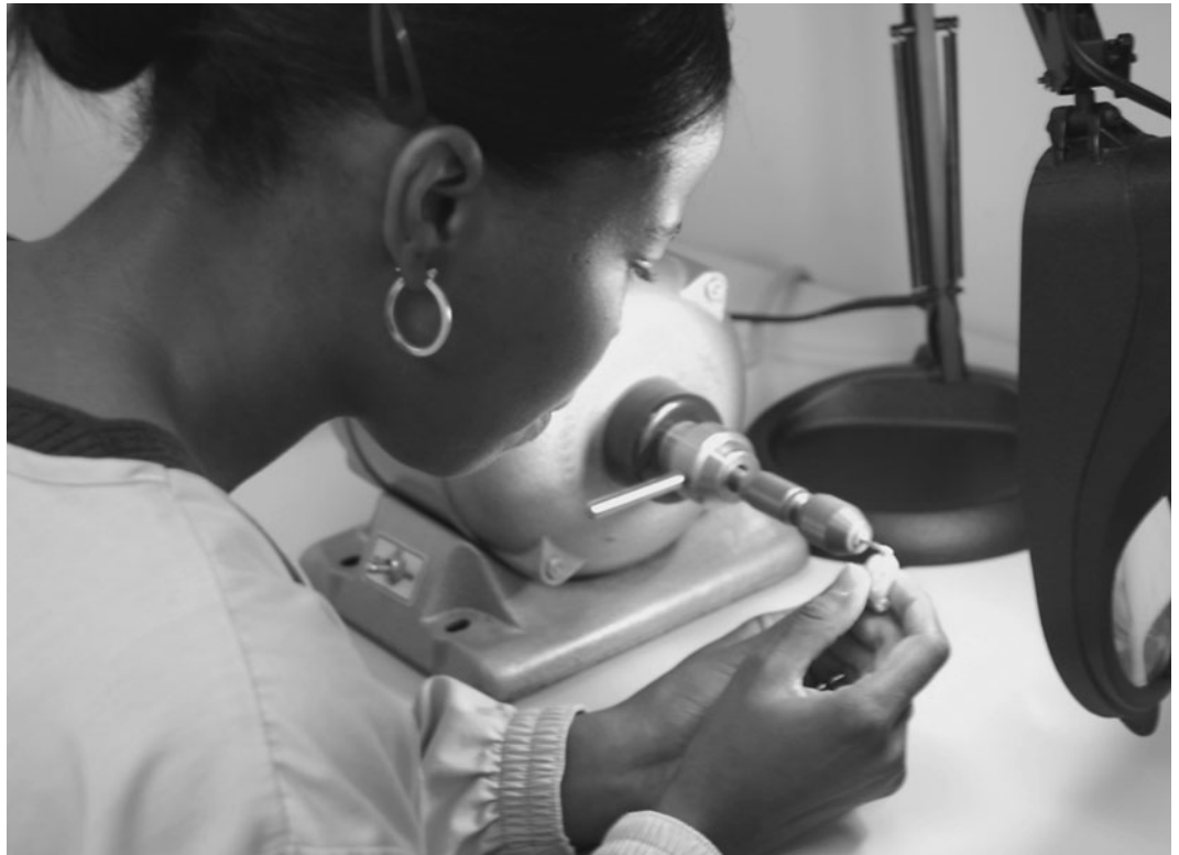
FIGURE 14.15 Earmolds and hearing aids can be ground and buffed when needed for greater physical comfort. The sound opening of the mold or hearing aid can be “belled” or scooped out to enhance high-frequency amplification and vent openings can be enlarged to decrease the amount of low-frequency amplification.
