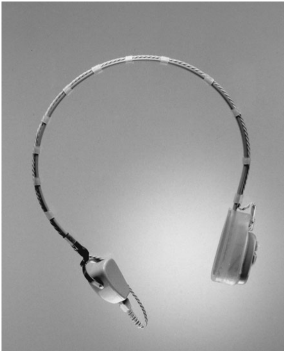
FIGURE 14.8 The vibrating receiver of a bone-conduction hearing aid sends sound waves to the cochlea through the bone-conduction auditory pathways of the skull. (Courtesy of Starkey Laboratories)
