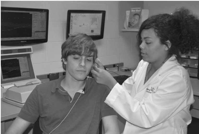
FIGURE 14.13 A soft silicone tube is placed in the ear canal near the tympanic membrane to obtain probe-microphone (real ear) measures of the acoustic characteristics of the hearing aid as worn.
