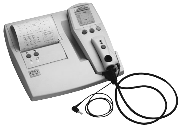
FIGURE 7.8 Commercial device for measurement of otoacoustic emissions, sounds generated by the cochlea indicative of cochlear function. (Courtesy of Grason-Stadler Co.)
