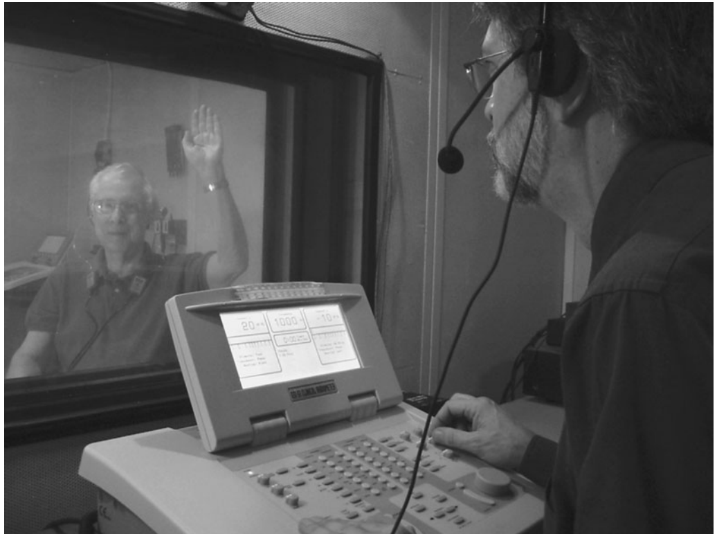
FIGURE 4.3 A commercial double-room sound-treated audiometric test chamber in use.
