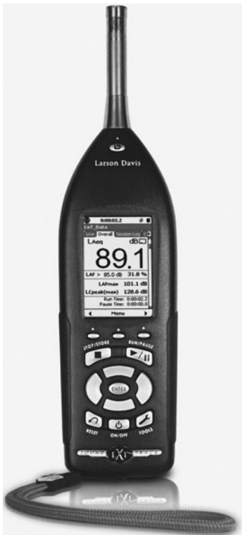
FIGURE 3.13 A commercial sound-level meter designed to measure the sound-pressure levels in various acoustical environments. (Courtesy of Larson-Davis Laboratory, a Division of PCB Piezotronics, Inc.)
