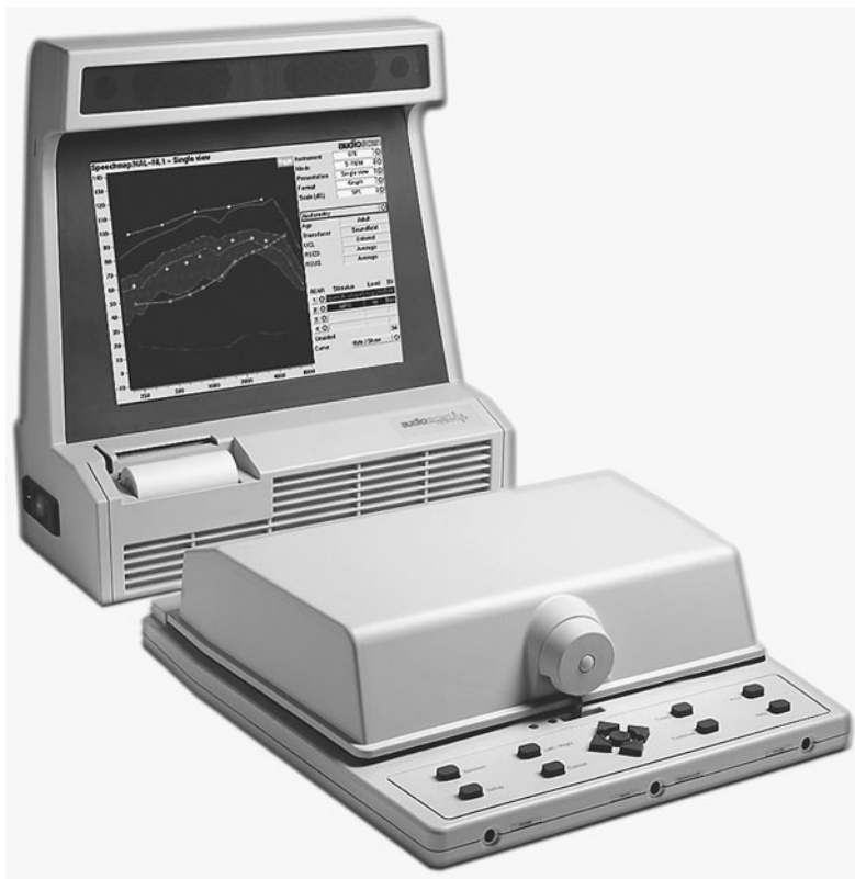
FIGURE 14.3 Hearing aid test system including sound chamber for 2\text{ cm}^3 electroacoustic analysis of hearing instruments and probe-microphone measurements. (Courtesy of Audioscan)
