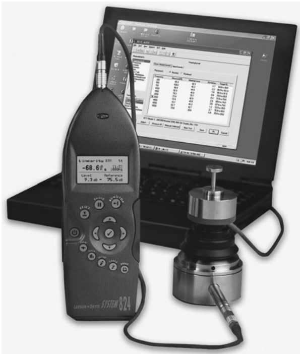
FIGURE 3.27 A commercial audiometer calibration device. A supra-aural earphone is placed on an artificial ear for calibration. A separate, smaller-sized, artificial ear is used for calibration of insert receivers. (Courtesy Larson-Davis Laboratory, a Division of PCB Piezotronics, Inc.)
