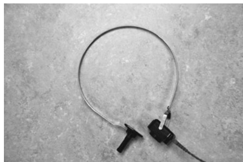
FIGURE 3.22 A bone-conduction vibrator through which pure tones may be routed using a pure-tone audiometer to measure bone-conduction sensitivity.
