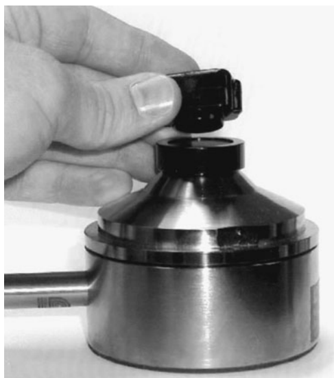
FIGURE 3.28 An artificial mastoid assembly for calibration of the bone-conduction system of an audiometer. The artificial mastoid has properties similar to the human skull, scalp, and skin. Here the bone-conduction vibrator of an audiometer is placed on the artificial mastoid, which will then be attached to the audiometer calibration device. (Courtesy Larson-Davis Laboratory, a Division of PCB Piezotronics, Inc.)
