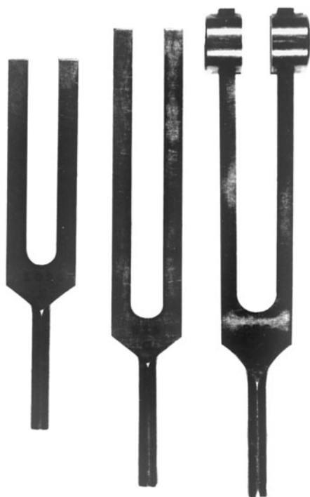
FIGURE 2.3 Several tuning forks. The larger forks vibrate at lower frequencies (produce lower-pitched tones) than the smaller forks.
