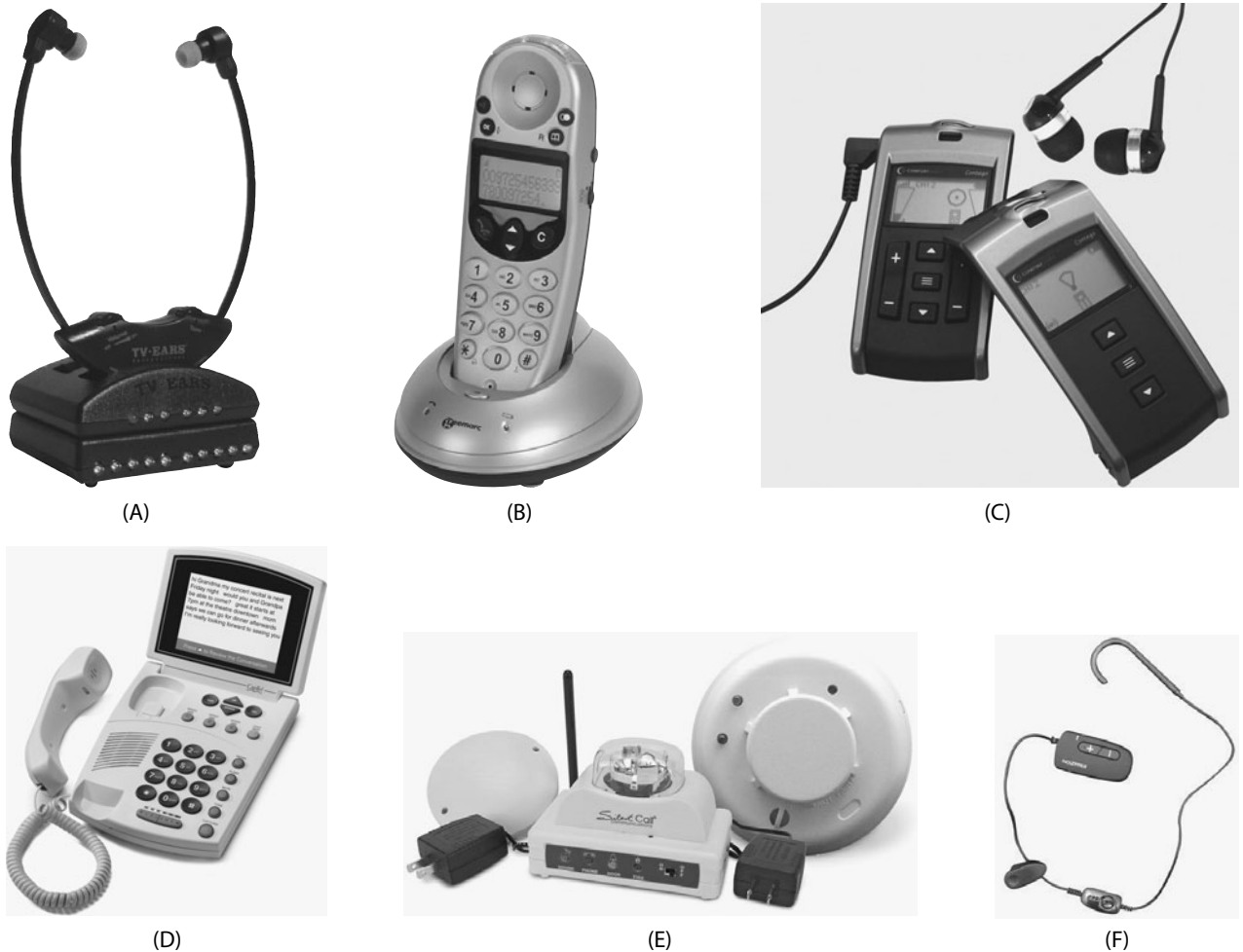
FIGURE 14.16 Examples of a few hearing assistance technologies for use by individuals with hearing impairment: (A) an infrared system for transmission and reception of auditory signals through invisible light frequencies, useful for the TV and in many live theaters and cinemas; (B) amplified cordless phone with caller ID; (C) FM system with microphones in both the transmitter and receiver for increased auditory signals, shown with earphones but also available with a neckloop that interfaces with hearing aid telecoils; (D) captioned telephone with text display used with the relay service; (E) smoke detector system that activates a bed vibrator for vibrotactile alerting; (F) amplified neckloop that picks up Bluetooth signal from a cell phone and creates an induction signal for the hearing aid telecoil. (Courtesy of beyondhearingaids.com)
