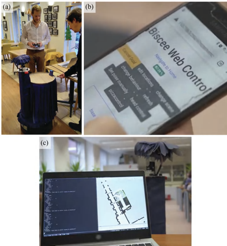
Figure 2.4 (a) Biscee is controlled by the human experimenter; (b) Biscee has a few pre-programmed actions that are displayed on command by the experimenter; (c) Biscee is moving autonomously in a room.
