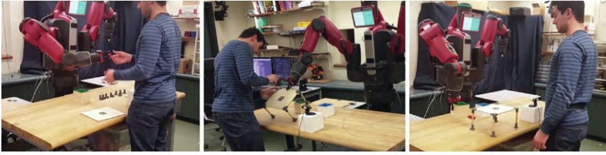
Figure 2.29 Snapshots acquired during the collaborative assembly of the table by a naive human subject and Baxter robot. (1) Baxter provides the tool to the participant; (2) the robot supports the human by holding the tabletop while the human screws the leg in place; (3) the user has finished his task and observes the robot freeing the workspace from the box of linkages. Such experiments are important for finding out how to organise the physical and communicative interaction between the two participants, but it can also be seen that the actual level of performance of the team is very low compared to working alone or a team of two humans (from Mangin et al., 2022).
