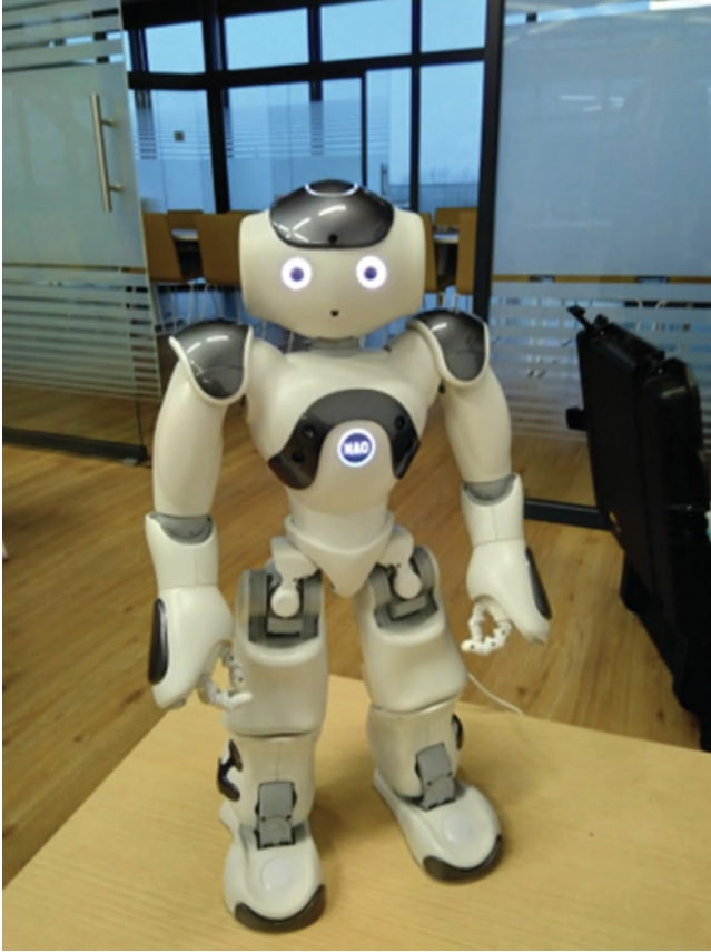
Figure 4.1 Photo of NAO, version 6. The robot shown in the picture is used for conducting social psychology HRI experiments by the Digital Interactions Research Group at the University of Debrecen, Hungary.
