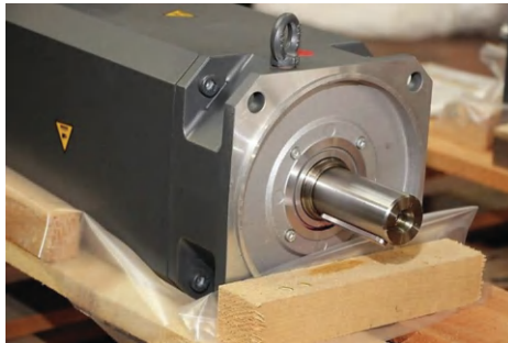
Figure 3.19 A typical servomotor used for controlling movements in robots (photo by Kitmondo PPM, Flickr).
