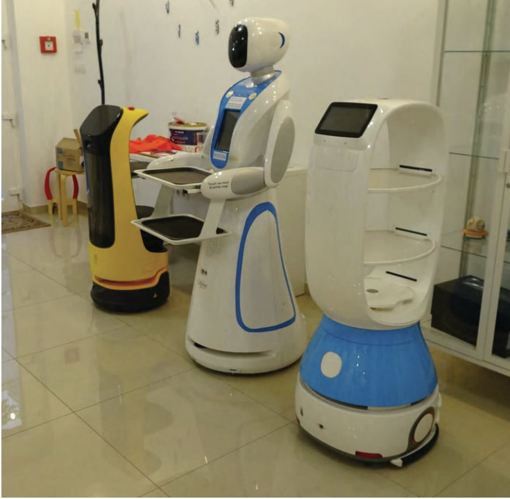
Figure 4.17 Examples of waiter assistant robots in the coffee shop of the Enjoy Robotics Company, Budapest, Hungary. From left to right: KettyBot by PUDU Robotics, Amy by Suzhou Pangolin Robot Corporation (Csjbot), and T1 dinerbot by Keenon.
