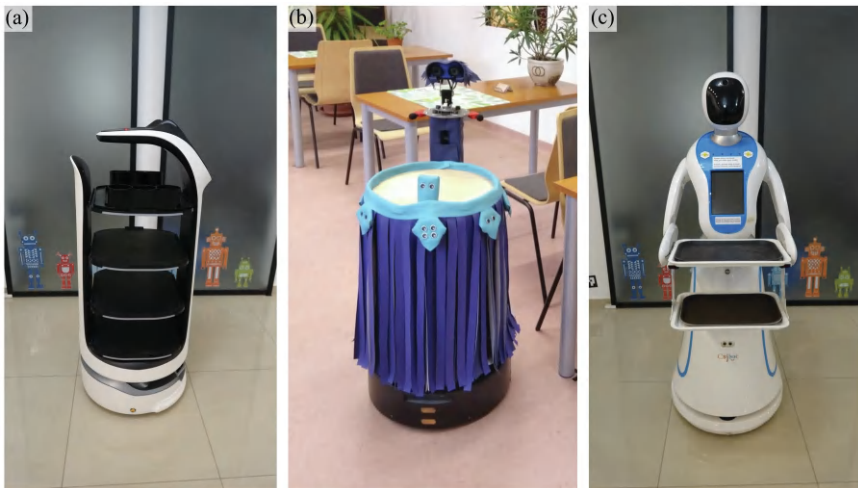
Figure 2.1 Waiter robots have different embodiments from resembling simple moving trays (although often having a screen with face-like touch screen), e.g., (a) BellaBot by Pudu Robotics; having more complex features such as a moveable head and/or extremities, e.g., (b) Bisce robot developed by the HUN-REN - ELTE Comparative Ethology Research Group, Hungary; or having humanoid form, e.g., (c) Amy service robot by Suzhou Pangolin Robot.
